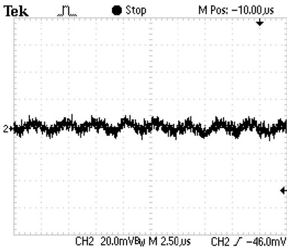
SW Noise (V<sub>IN</sub>=3.6V, I<sub>LOAD</sub>=100mA)
